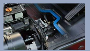
1. In addition to rubber damper between overhead and frames, compound engine damper and full floating power train achier flexible connection between frames and driving system, as a result, traveling vibrations and vibrations from the driving system are significantly reduced.
